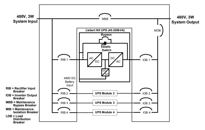
Figure 15 Paralleling cabinet with input and bypass circuit breakers
